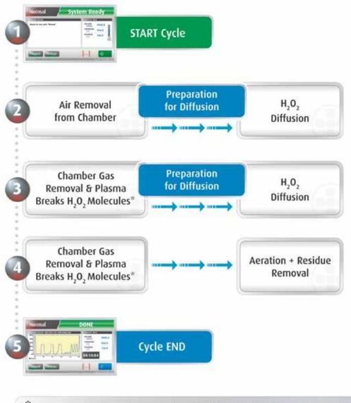
Plasma breaks down Hydrogen Peroxide (H<sub>2</sub>O<sub>2</sub>) molecules into Water (H<sub>2</sub>O) and Oxygen (O<sub>2</sub>) outside the chamber
