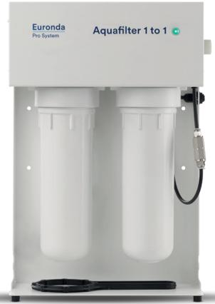
Device for the production of deionised water for autoclaves, in accordance with EN 13060 (<math>< 15 \mu\text{S}/\text{cm}</math>). Only one Euronda Pro System autoclave can be supplied. It deionises on average 1 litre of water per minute. It can be equipped with automatic shut-off device. It can be placed directly on the worktop or inside a cabinet, as well as mounted to a wall. Included in the initial equipment are two ion exchange resins.
