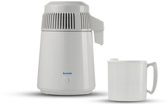
Water distiller for obtaining distilled water by boiling and subsequent steam condensation. It distils 0.7 L of water per hour. 4-litre capacity. It fulfils the safety and electromagnetic compatibility (2014/30/EU) and low voltage (2014/35/EU) tests.
